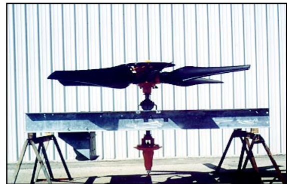
Inverted Actuator-Variable-Pitch Fan Fig. 15
